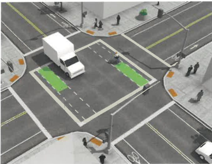
Figure 57 Intersection crossing markings
